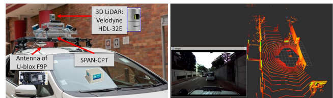
Fig. 3 Left: Setup for the sensor platform. A u-blox F9P, Velodyne HDL-32E 3D LiDAR, and ground truth positioning provided by SPAN-CPT are adopted during the evaluation. Right: The typical urban environment of Hong Kong to be evaluated.
